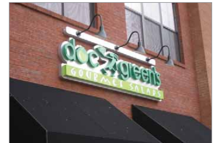
Signage shall be externally lit, except that signage within the shopfront glazing may be neon lit
