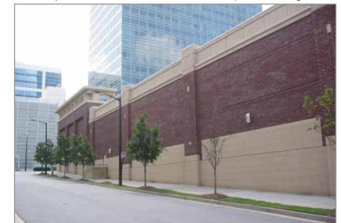
✗ Windows shall be a minimum of 15 percent of the total surface wall area along facades that do not face streets (excluding outbuildings).
