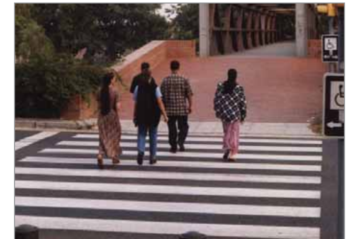
"Piano striped" crosswalk on Secondary Streets
