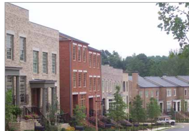
✓ No more than three adjacent attached or detached single-family houses should have the same roof form
